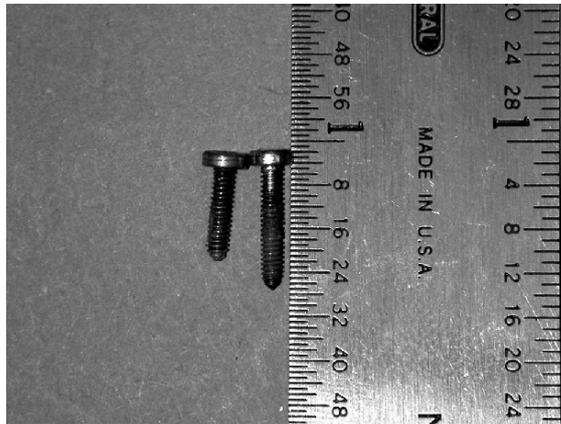
*NOTE: Screw torque should be set at 16 Ncm +/-2 Ncm. This can only be achieved with a properly calibrated torque driver. All torque drivers should have routine inspections for correct calibration and proper performance.*
